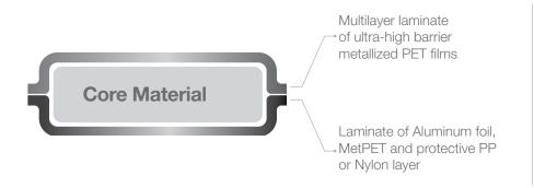
The hybrid solution: Pair the foil layer with the high-temperature side, and the metallized laminate to the cooler-facing side.
