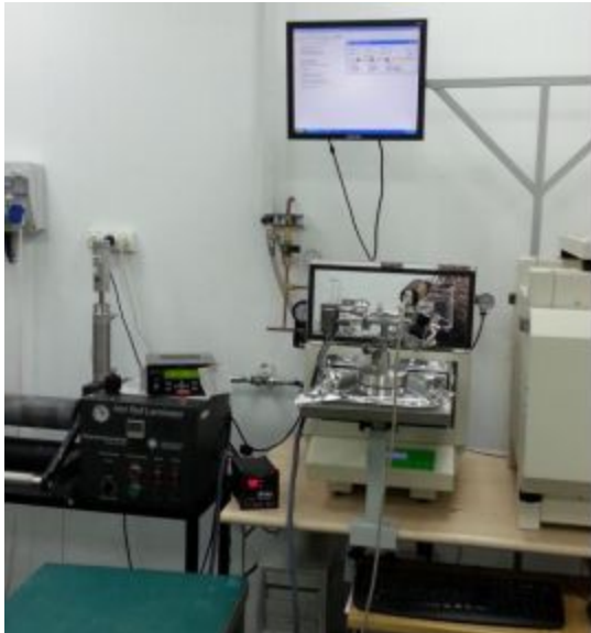
Figure 1(b) Sample inside thermal conductivity measurement device (LaserComp FOX314)
