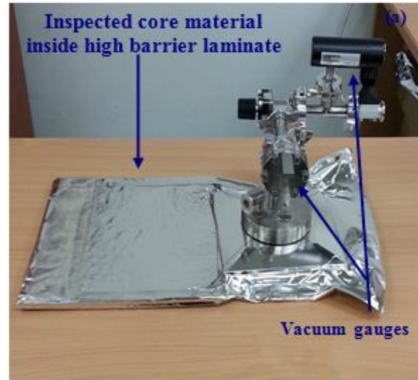
Figure 3(a): The \lambda vs P system for core material experimental characterization
