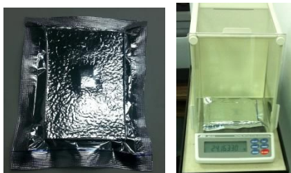
Figure 9(a): small panel (~15cmx12cm) with glass fiber and desiccant (b): Weighing the panel with an analytic balance
